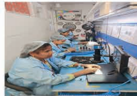
Clean Room Booth for Lens Assembly (Class 8)
