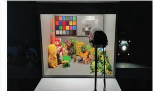
Dark Room Camera Tuning and Validation
